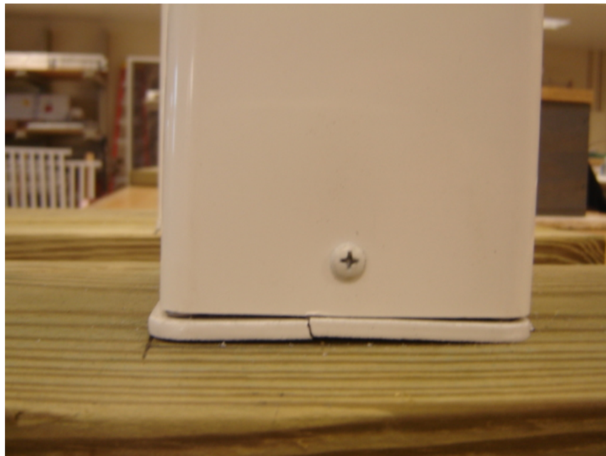
Photo No. 4 Uplift Resistance Tests - Plate Failure
