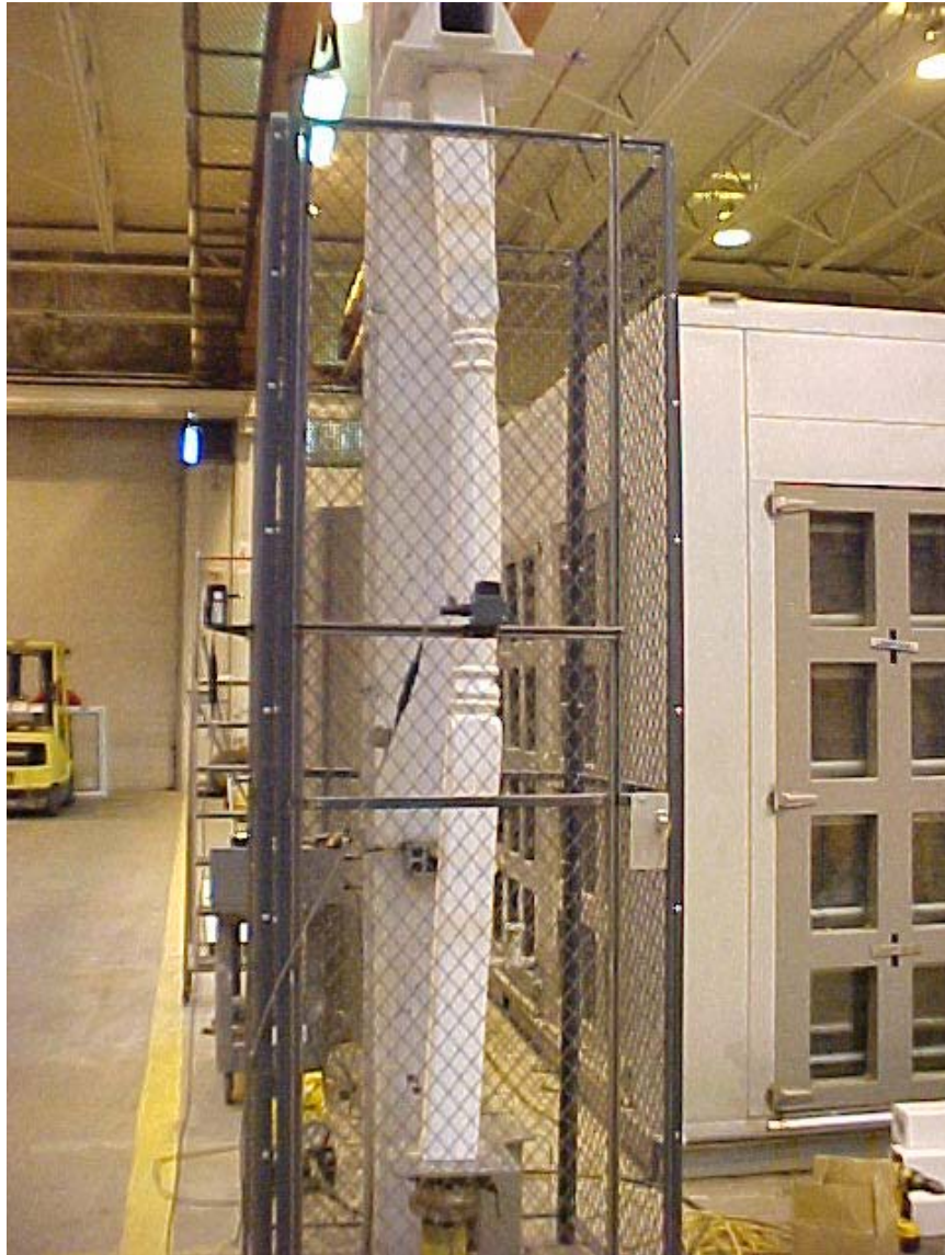
Photo No. 2 Axial Compression Load Test in Progress
